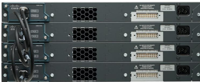
Figure 2. Cisco FlexStack Switch Stack
