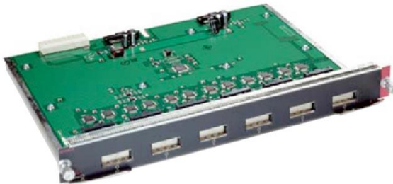
Figure 22. WS-X4306-GB Cisco Catalyst 4500 Gigabit Ethernet Module, 6 Ports (GBIC)
