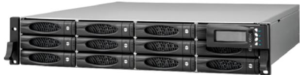
The EP-2123 series RAID subsystem features 6Gb SAS or 8Gb FC-AL host performance to increase system efficiency and performance. It features high capacity expansion, with 12 hot-swappable SAS2/SATA3 hard disk drive bays in a 19-inch 2U rackmount unit, scaling to a maximum storage capacity in the terabyte range. The EP-2123D series also supports dual controllers which provide better fault tolerance and higher reliability of system operation.
