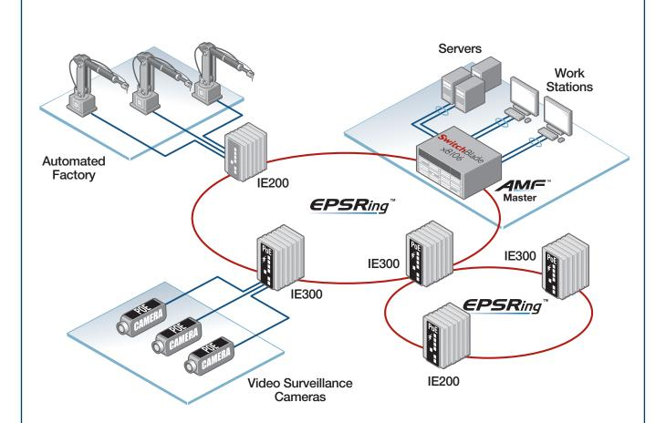
Ethernet Protection Switched Ring (EPSRing™) and ITU-T G.8032 provide high speed resilient ring connectivity; this diagram shows the IE Series in a double ring network topology.
