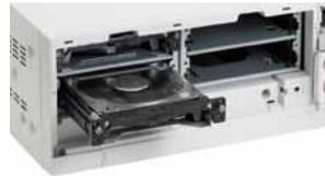
Maintenance friendly HDD installation from the front panel
