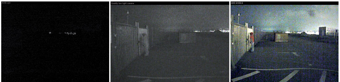
Lightfinder technology with AXIS Q1602/-E, AXIS Q1614/-E Network Cameras Left: Reference image, Middle: High-end surveillance camera, Right: AXIS Q1602/-E Network Cameras
