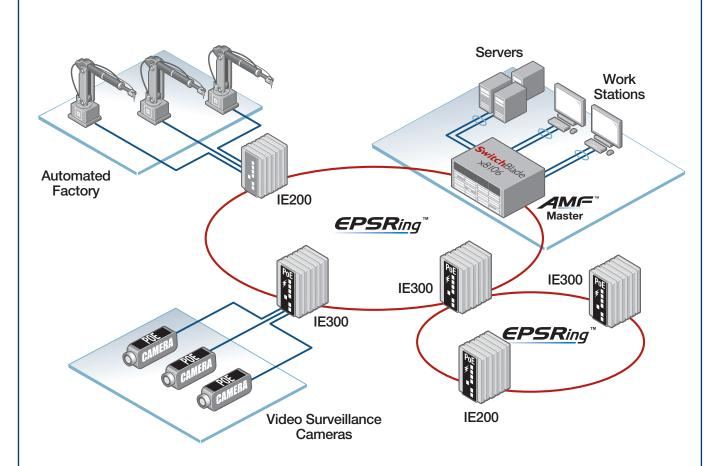
$\label{eq:connectivity:provide} EPSRing^{TM}\ ITU-T\ G.8032\ provide\ high\ speed\ resilient\ ring\ connectivity;\ this\ diagram\ shows\ the\ IE\ Series\ in\ a\ double\ ring\ network\ topology.$
