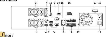
The rear panel of DS-9016HUHI-K8 provides 16 video input interfaces.
