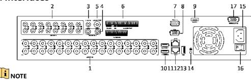
The rear panel of DS-9024HUHI-K8 provides 24 video input interfaces.
