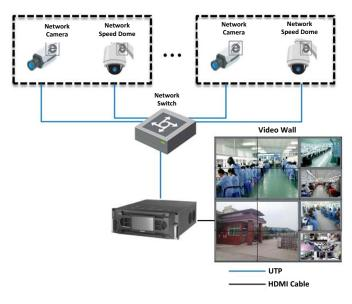
Note: The /H and /H/I models provide 12 HDMI outputs for video wall display.
