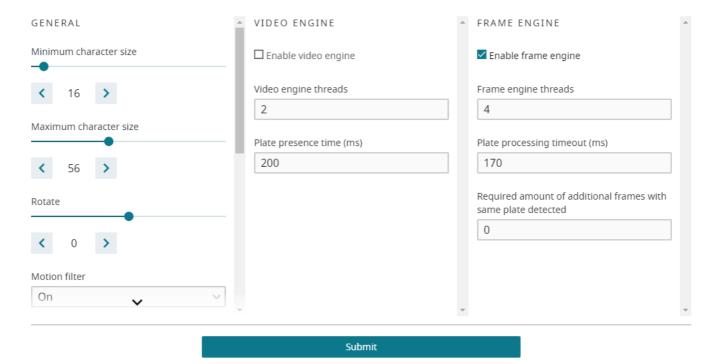
Choose your desired recognition parameters and click *Submit* to add the channel into LPR configuration. If the target Luxriot EVO server is online and reachable, the channel analysis will be started immediately. You can add one or more channels from every connected Luxriot EVO server for a single LPR server to work with. To edit or delete existing channel, simply click the corresponding controls on the right of the channel name in the list.
