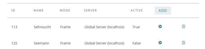
If there are multiple channels in the list, you can quickly track their current operation by looking at the **activity status**: the channels available and enabled for recognition will have the status saying *True*, and those unavailable or with processing disabled will be marked as *False*.
