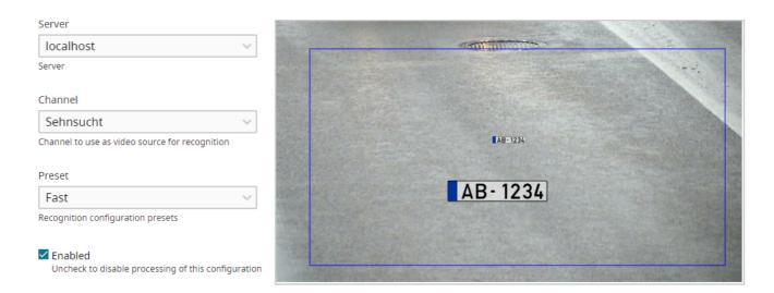
Select a server from the list of your connected servers and then select one of the channels. Note that channel must be enabled in Luxriot EVO server configuration and the server itself must be connected in LPR. If the Luxriot EVO server is offline, you will be unable to select it in the *Add new channel* form: in such case, ensure Luxriot EVO server availability and try adding the channel again.
