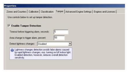
Once enough of the image has changed and remained so for a certain length of time, a tamper alarm is triggered.
