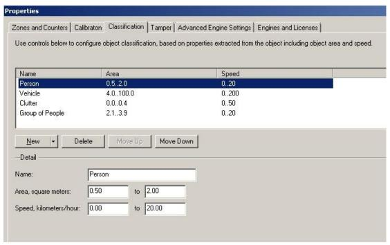
Adjust the minimum and maximum object speed and area, and apply the changes.
