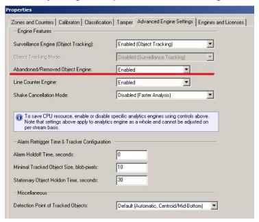
**NOTE:** The algorithm used for abandoned and removed object detection is the same in each case: it cannot differentiate between abandoned or removed objects. This is a fundamental limitation of the algorithm and arises because it just analyses how blocks of pixels change with respect to a background model that is constructed over time. When an object is inserted into the background (abandoned) it looks the same to the algorithm as when an object is removed from the background.
