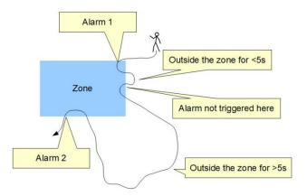
In this case, an alarm is not raised when the person enters the zone for the second time, because the time between the occurrence of the last alarm of the same type for the object is less than the Alarm Holdoff Time. When the person re-enters the zone for a third time, the elapsed time since the previous alarm of the same type for that object is greater than the Alarm Holdoff time and a new alarm is generated.
