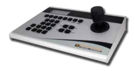
Via RS-485 interface, the PLANET CAM-KB300 is a 3-Axis Control Keyboard which provides upward, downward, leftward, rightward, clockwise and counterclockwise with the joystick. It can remotely control the external scanners, speed dome cameras and PTZ receivers, and offers long distance control up to 4000 feet.
