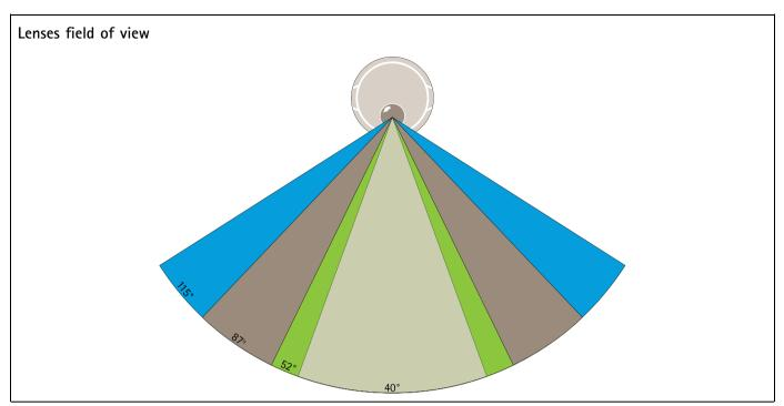
Standard lens field of view: 87°. Optional lenses field of view: 2.8 mm: 115°, 6 mm: 52° and 8 mm: 40°.
