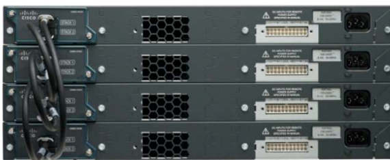
Figure 3. Cisco FlexStack Module and Switches
