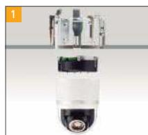
Install the ceiling bracket (option) on the ceiling, and screw the camera's ceiling mount section onto it at 3 points.
