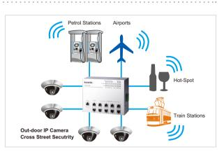
monitoring, or WiMAX systems for internet access in train stations, airports or Hot-spots. Moreover, the 8 PoE ports of JetNet 5710G integrate forced powering mode function to drive the legacy Powered devices, which does not comfort to the IEEE 802.3 PoE standard. The additional dual Gigabit ports provide more resilient and redundancy for users while forming a ring network and delivering increased bandwidth to the central network.
