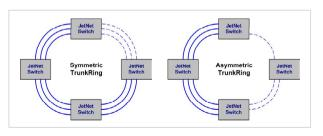
redundancy at different locations in accordance to the need. The link with less speed is more likely to be used as the backup path for restoring the network to full play capacity.
