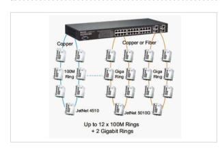
The JetNet 5728G series supports the new generation ring technology – MSRTM which includes various new technologies for redundancy applications and structures of different networks. The PoE switch allows to aggregate up to 14 Rapid super rings, including 12 Fast Ethernet plus 2 gigabit Ethernet Rings. With the MSRTM technology, a node can be configured to multiple rings with the failover time in as little as 5ms and zero-second of restoration time.
