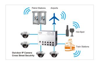
direction control for cross—street monitoring, or WiMAX systems for internet access in train stations, airports or Hot-spots. The additional dual Gigabit ports provide more resilient and redundancy for users while forming a ring network and delivering increased bandwidth to the central network.
