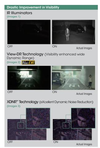
\*1 0 Ix requires the use of IR illuminators. IR rays are not visible to the human eye. When the IR illuminators is activated, the image is in black and white.
