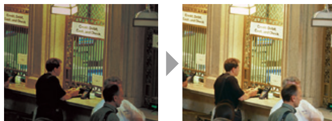
■ F/1.4 ■ F/1.0 F/1.0 lens has two times light gathering power compared to F/1.4 making a 1 lux camera sensitivity into a 0.5 lux sensitivity.
