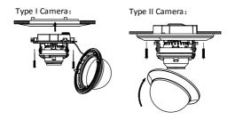
Figure 2. 8 Fix the Camera to the Mount
