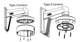
Figure 2. 6 Attach the Base Plate to the Bracket
