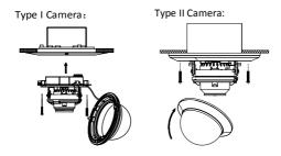
Figure 2. 10 Fix the Camera to the Junction Box
