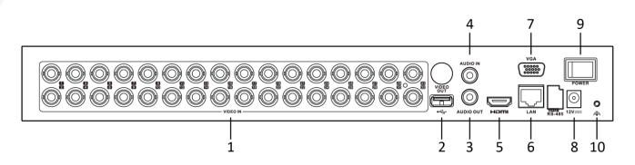
\*: The rear panel of DVR-216/224G-K2 provides 16/24 video input interfaces. DVR-216G-K2 provides 2 USB 2.0 interfaces at rear panel, but no USB interface at front panel.
