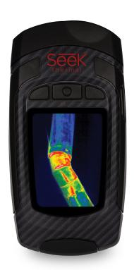
RevealPRO is our most advanced handheld thermal imaging camera yet. Highly durable and easy to use, RevealPRO combines a high-performance 320 x 240 thermal sensor with intuitive software to help you work smarter. And, when you need it, a powerful 300-lumen LED light is available at the touch of a button. Offering adjustable thermal span, level, and emissivity settings, the RevealPRO delivers unprecedented high-resolution thermal imaging and software capabilities available at this price.
