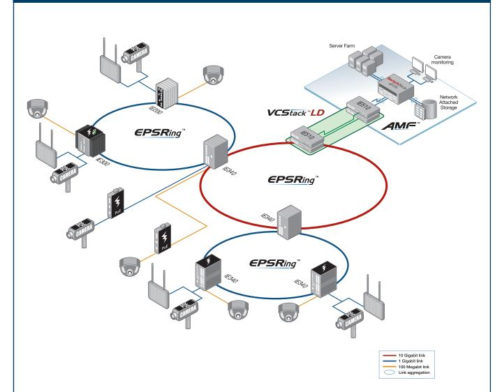
EPSRing<sup>™</sup> and ITU-T G.8032 provide high-speed resilient ring connectivity. This diagram shows the IE Series in a double ring network topology.
