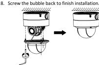
Figure 2-24 Finish Installation
