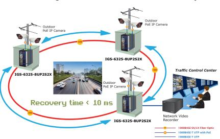
ERPS Ring for Video Transmission Redundancy
