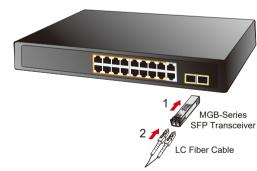
Figure 5-3: Plug In the SFP Transceiver
