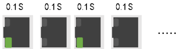
Figure 2.5 - PoE Over Current LED Sequence
