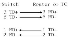
Straight Through Cable Schematic
