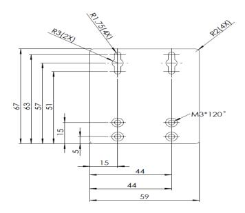
Figure 3.5 - Wall Mounting Bracket Dimensions
