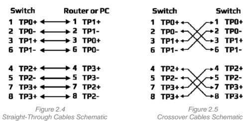
The following figures show the 10,100, and 1000 Ethernet RJ-45 pin outs.
