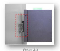
Stable the Switch on DIN-Rail
