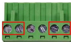
Figure 2.13 - Power Terminal Block
