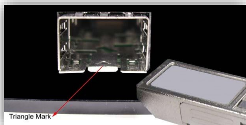
Figure 2.7 - Transceiver to the SFP Module
