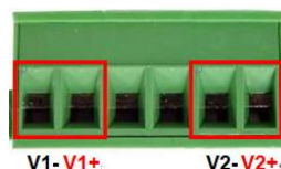
Figure 2.12 - Power Terminal Block
