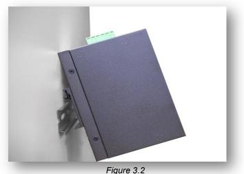
Insert the Switch on the DIN-Rail
