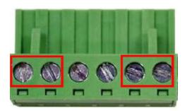
Figure 2.15 Power Terminal Block
