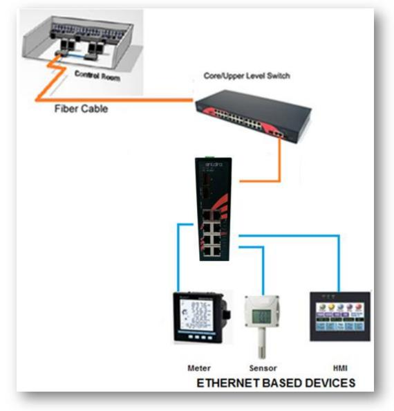
Figure 5.1 Industrial PoE Ethernet Switch Application Reference
