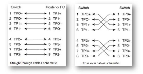
Figure 2.7 Straight-Through Cable Schematic
