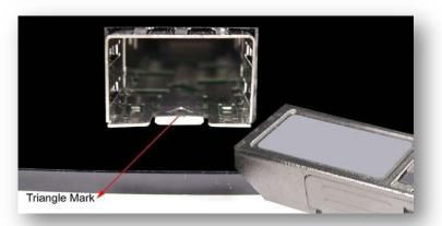
Figure 2.9 Transceiver to the SFP Module
