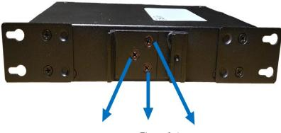
Figure 3.4 Remove DIN-Rail Bracket from the Switch
