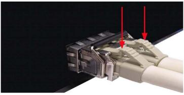
Figure 2.12 Remove LC Connector
