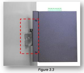
Stable the Switch on DIN-Rail
