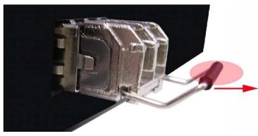
Figure 2.13 Pull Out from the SFP Module
