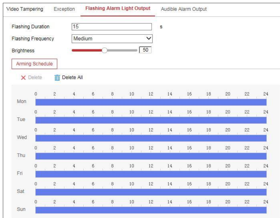
Figure 10-9 Flashing Alarm Light Output Settings
