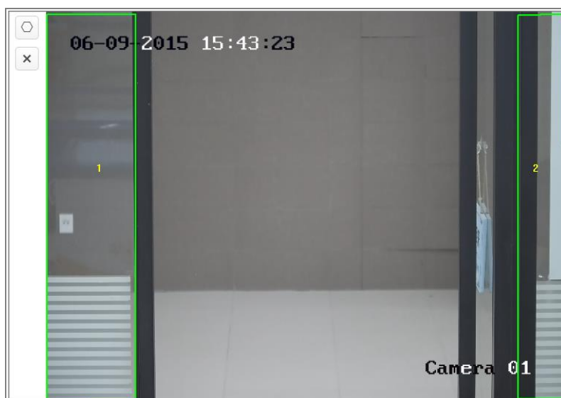
Figure 10-30 Draw Shield Area
